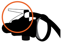
Extinguisher handle Use to activate the suppressant and make selections in the launcher and headset.
