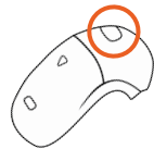
Hose tracker teleport and interaction button Use to activate the headset VIVE menu, the launcher, scenario selection and teleport function.
