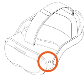
Headset side button Press and hold button to return to lobby. Double-press to switch to pass-through mode which enables visibility of real world.
